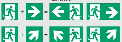
Supplementary arrow sign (type D of ISO 3864-3) in white on green to be used to give directional information (direction examples, the arrows may be rotated in increments of  $45^{\circ}$ ). You can mix signs according to examples above.
