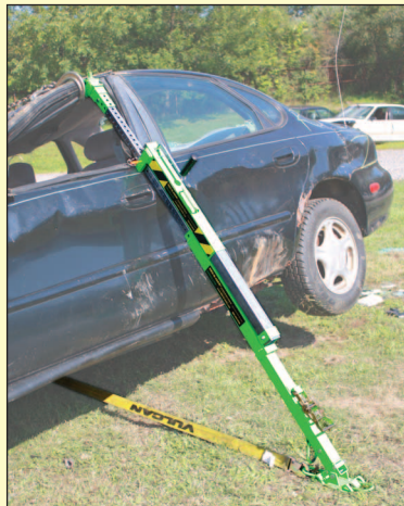
Add-on Jack Engages Without Pinning for Quick Lifting Ability
