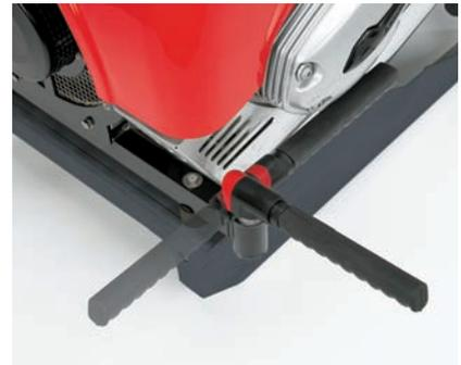
FOX portable pump with swinging out carrying handles
