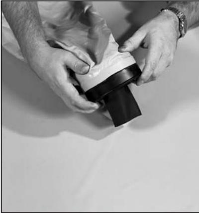
10. Lubricate the complete cuff with soapy water and insert it (from inside the suit) into the sleeve ring. Push it firmly into place. NOTE! Take care not to squeeze the suit material between the rings. Make sure the cuff ring is aligned straight before pushing it into place. To make it more comfortable for people with thick wrists, cut off an appropriate length of the cuff.
