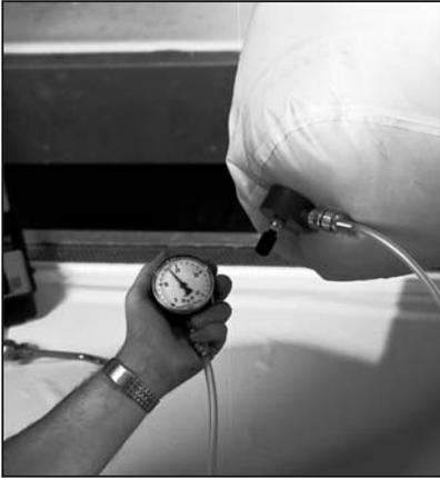
4. Close the zipper and connect the pressure gauge to the adapter.
