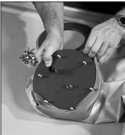
3. Unscrew the nuts on the face seal plate and detach the top ring. Place the plate under the face seal (insert from inside). Adjust the face seal so that it covers the outer part of the plate without being in contact with the screws.
