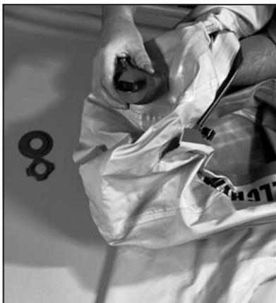
2. Install the blind plugs in the other exhaust valves. For old suits with grey exhaust valves there is a small plug available - please contact your distributor.
