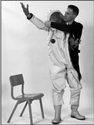
4. Put right arm into the suit and hump over the breathing apparatus.
