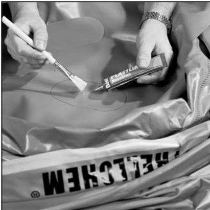
4. Apply a thin layer of the glue to the damaged area and...
