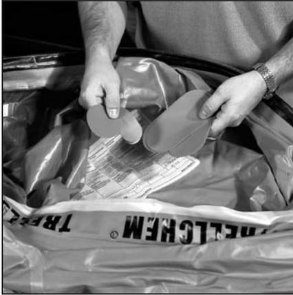
2. Select a patch which is large enough to cover the damage with a margin of at least 15 mm around the damage. Position the patch accordingly and mark the position with a pen.
