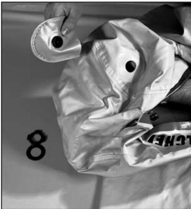
1. Remove one of the exhaust valves and install the adapter.
