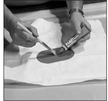
5. ...to the patch. Allow to dry 5-10 minutes, until it is tacky. **Important:** repeat the previous and this step, applying a second layer of glue. Let dry until tacky.
