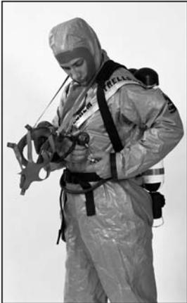
8. Connect the ventilation hose to the inlet-/regulating valve.
