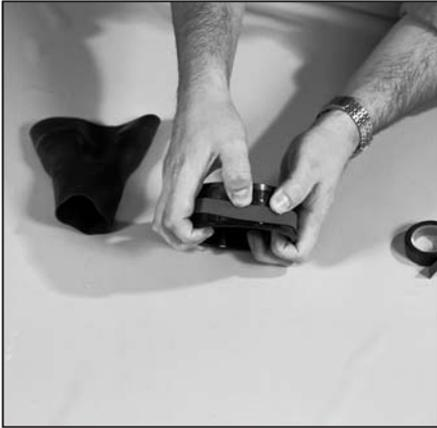
6. Place the rubber gasket around the thicker half of the cuff ring. Push it so that it is positioned immediately next to the ridge at the end of the ring.
