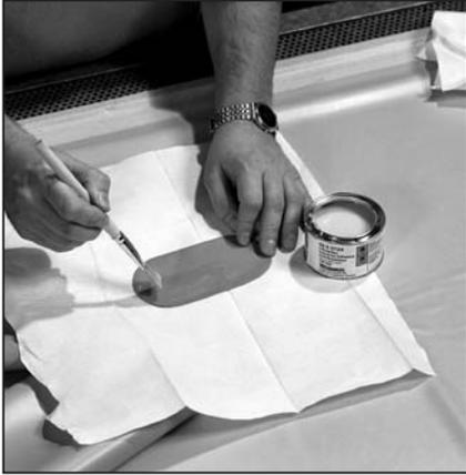
6. ...to the patch. Allow to dry 5-10 minutes, until it is tacky. **Important:** repeat the previous and this step, applying a second layer of glue. Let dry until tacky.
