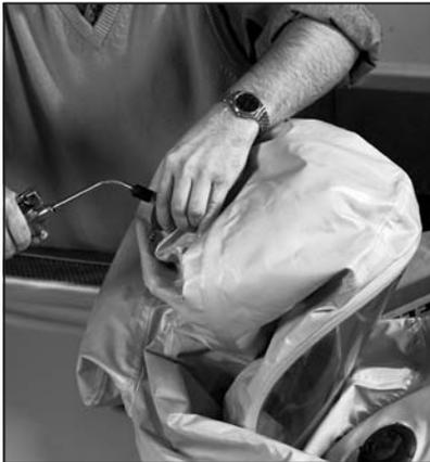
5. Inflate the suit through the valve on the adapter. Test the suit as described below.
