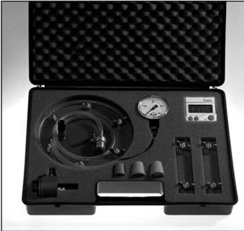
1 pce face seal plate with connection nipple and valve (type T)
