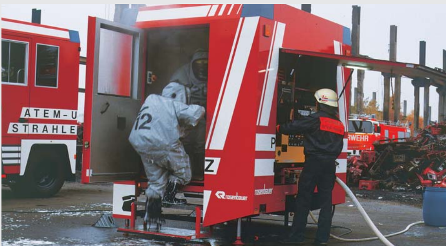
Breathing Air-Vehicle, which can split of the Decon-Unit
