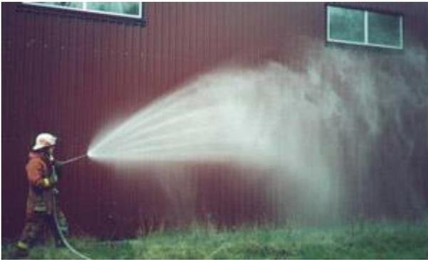
Fognail Attack has a trajectory length of 8 m
