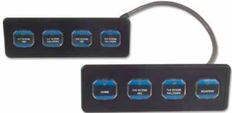
Two 6311-0400-00 connected with 0L40-2020-00 cable assembly
