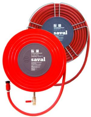
have a strong and rugged PUR powdercoating in the colour RAL3000. The drum is supplied with a high-quality semi rigid hose (¾" or 1" I.D.) approved to EN694 and a shockresistant adjustable nozzle (shut-off/fog/stream). The nozzle has a bore equivalent to a diameter of 7 or 10 mm.
