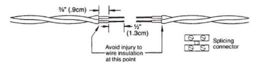
**Step.2**: Install wires as shown below making sure the entire 1/2" (1.3cm) portion of bare Linear Heat Detector conductor is embedded in splicing connector.
