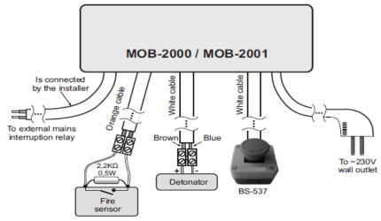
**<u>Note</u>**: Fire Detection-Suppression Panel MOB-2001 is compatible only with the Linear Heat Detection Cable supplied by MOBIAK.
