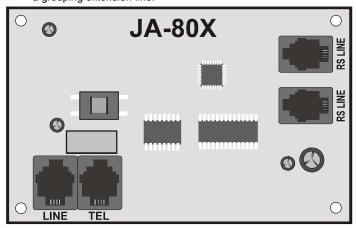
**Note:** The communicator must be plugged directly into a telephone line socket. All other devices should be connected to the communicator output marked TEL.
