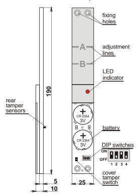
LED indicator - 15 minutes after closing the detector's battery cover, the LED indicates detector triggering (a flashing light indicates window opening, a long light indicates that both rear tamper sensors have been triggered).
