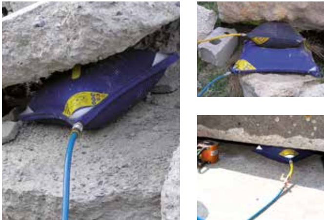
- thickness incl. profile of HLB 1/3/5 is 22 mm and of other models 25 mm - reflecting labels: HLB 1/3/5 on 1 corner; other models on 3 corners
