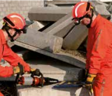
Power Wedge creates opening for lifting bag (see page 36)
