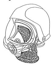
As well as at its upper side the visor has a snap-holder at the lower side.
