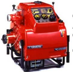
Engine 617cc Tohatsu 2 strokes, water-cooled gasoline engine Authorized output 40.8PS (30kW) Pump performance 1450 liter / min. at 0.4MPa 1000 liter / min. at 0.8MPa 600 liter / min. at 1.0MPa Dry weight 85kg
