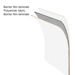
Strong and flexible polyamide fabric laminated on each side with a barrier film laminate.
