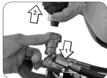
Whenever the SCBA is pressurised the coupling is firmly locked by the pressure and impossible to disconnect.
