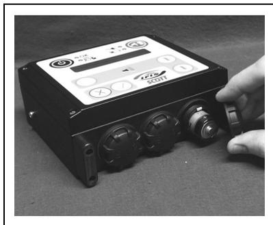
1. Using finger-pressure only, unscrew and remove battery compartment cover by turning in an anti-clockwise direction.
