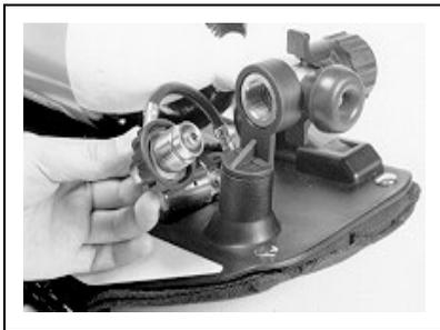
8. Check that the cylinder handwheel connector O-ring is clean and in good condition. Screw the cylinder connector firmly into the cylinder valve outlet.
