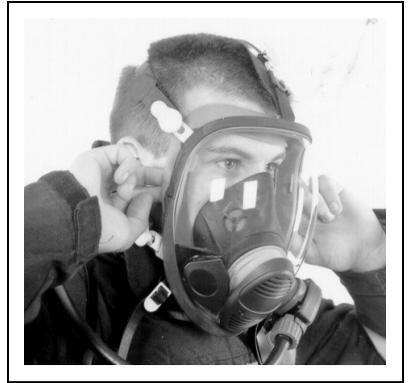
1. With the cylinder valve open, insert a finger under face seal and check for a steady outward flow of air. Remove finger and allow mask to re-seal.
