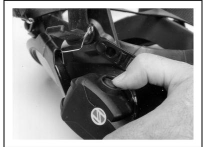
1. Press the black rubber reset button on the side of the DV and check that the red bypass knob is turned so that the flat on the bypass knob aligns with the DV outlet.
