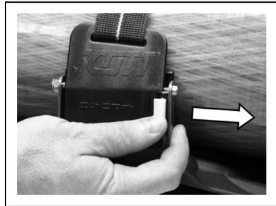
4. Use the thumb of your right hand to push the release tag away from the clamp mechanism in the direction of the arrow that appears on the moulded clamp cover. The clamp mechanism will open, allowing the cylinder nearest to the clamp to move freely within the cylinder band.
