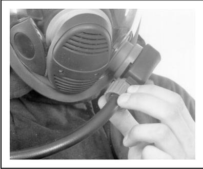
1. With the cylinder valve closed, open the bypass knob briefly to vent air from the system.
