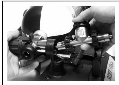
6. Manoeuvre the cylinder valve end of the remaining cylinder to allow removal of the **Duo** manifold from the cylinder valve retainers.
