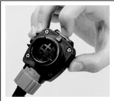
2. Check that the orange O-ring on the DV outlet is clean and in good condition.
