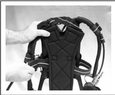
7. Pass the excess cylinder band between the backplate and backpad, at the point where the centre-straps retain the pad to the backplate.
