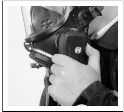
1. Check that the flat on the DV bypass knob aligns with the DV outlet and press the black reset button.
