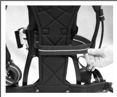
8. Route the cylinder band around the backpad and insert the end of the band between the backplate and backpad.
