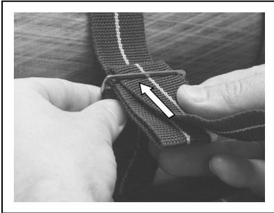
8. Holding the flag-end loop and cylinder band together, feed through the buckle on the cylinder dividing loop. The cylinder will move freely within the cylinder band.
