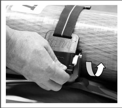
18. Apply gentle pressure to the clamp mechanism by pushing downwards and toward the cylinder to close the mechanism and tighten the cylinder band. The clamp mechanism will lock automatically when closed.
