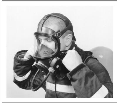
2. Tighten harness side straps. DO NOT over-tighten.
