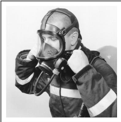
2. Tighten harness side straps. DO NOT over-tighten.
