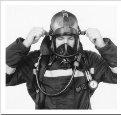
2. Adjust the facemask top strap so that the mask is at the correct level with the face and the head-harness pad is in the centre of the back of the head, then tighten harness straps in sequence, **Bottom, Middle, Top**. DO NOT over-tighten.
