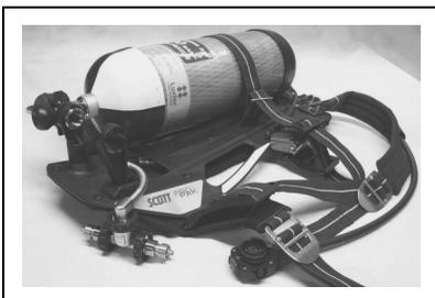
10. Slide a fully-charged cylinder along the backplate and through the loosened cylinder band. Position the cylinder outlet through the cylinder valve retainer.
