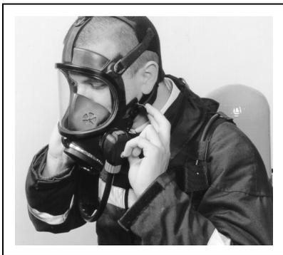
2. Release the head-harness by pulling the harness buckles forwards. Remove mask and let it hang from the neck strap.
