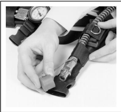
1. Check the supply airline flow and pressure. Remove connector dust caps and check for wear and damage.
