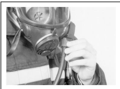
2. Turn on the DV bypass knob and check for a steady flow of air into the mask. Close the bypass knob.
