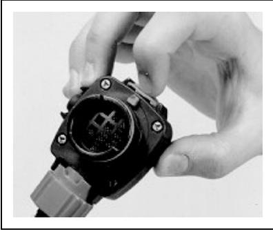
1. Operate the DV locking catch and bypass knob several times and check that they do not stick. If either is not free moving, attach explanatory note and return for service.
