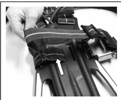
9. Ensure that the redundant cylinder band dividing loop (arrowed) lies flat against the backplate, in preparation for single cylinder fitment.
