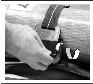
7. Apply gentle pressure to the clamp mechanism by pushing downwards and toward the cylinder to close the mechanism and tighten the cylinder band. The clamp mechanism will lock automatically when closed.
