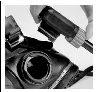
3. Fit the DV to the facemask and check that the red locking catch engages fully. Twist the DV gently to confirm that it has.
