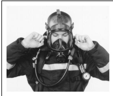
1. With the cylinder valve open, insert a finger under face seal and check for a steady outward flow of air. Remove finger and allow mask to re-seal.
