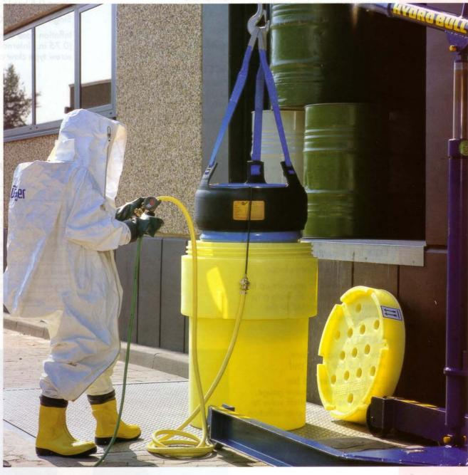
Lifting and sealing damaged drums into a safety container could not be easier or gentler. No matter how cramped the space, the Vetter Pneumatic Lifting Sleeve can extract any drum from among others in storage.
