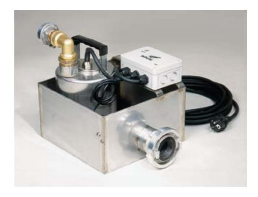
The Drainage pump is used for pumping the water from the tent into a wastewater container or the sewage system if the water is not contaminated. It is of type rotation pump in stainless steel with integrated water level switch. This allows the pump to work automatically as soon as the water in the shower tent has reached a level of 40 mm.
