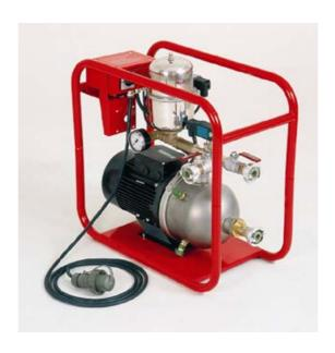
The Water pump is used for delivery of water to the showers in case a public water system not is available and when no Air Heater is used. It is of type horizontal centrifugal pump. It is pressure controlled with switch-on / off pressures at approx. 2,5 and 4,5 bar. The electric cable is equipped with safety plug.
