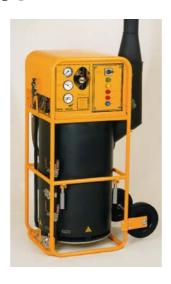
The flow heater is a two-stage heater that at the same time supplies two different outlets with thermostatically controlled water. It can be carried by means of 4 handles or driven by means or 2 wheels. It uses either diesel oil or petrol for heating plus electricity.
