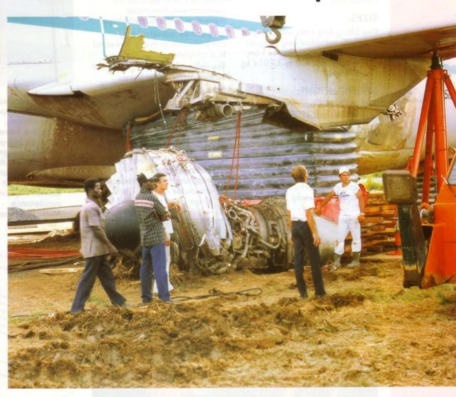
We call these bags the gentle giants, since they do a powerful lifting job at an operating pressure of no more than 0.5 bar (7.25 psi). Vetter Aircraft Lifting Bags raise aircraft back onto their legs after crash-landings off the runway, or when their landing gear buckles leaving them belly-flat, helplessly spreadeagled on the ground. They need at most 20 cm (7.9 in.) to be
