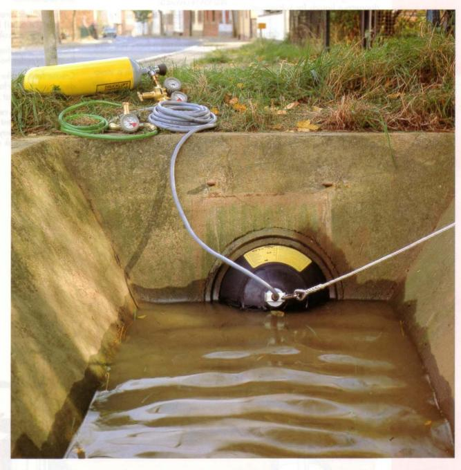
These bags are ideal for running leakproof tests with reduced bracing on water mains, at a backpressure of 0.5 bar (7.25 psi) or 1.0 bar (14.5 psi). Should toxic gases or liquids seep
